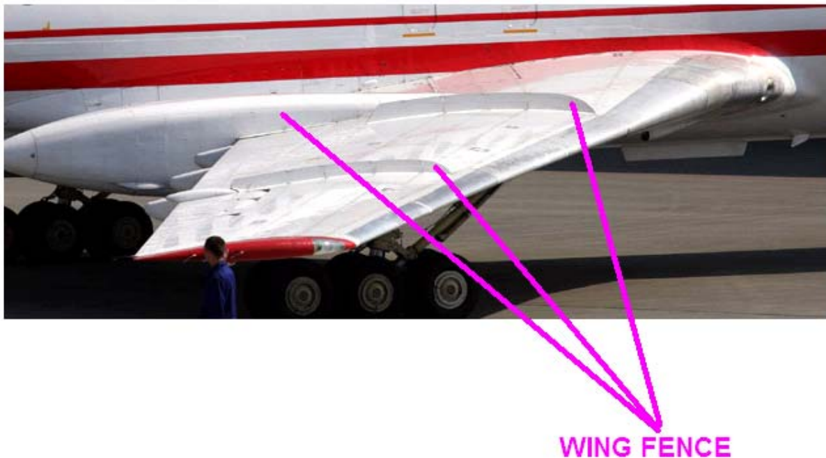
Fig. 17. The wing fences of the TU-154 shown for P101. These are not present on the model used by [1], [6].
